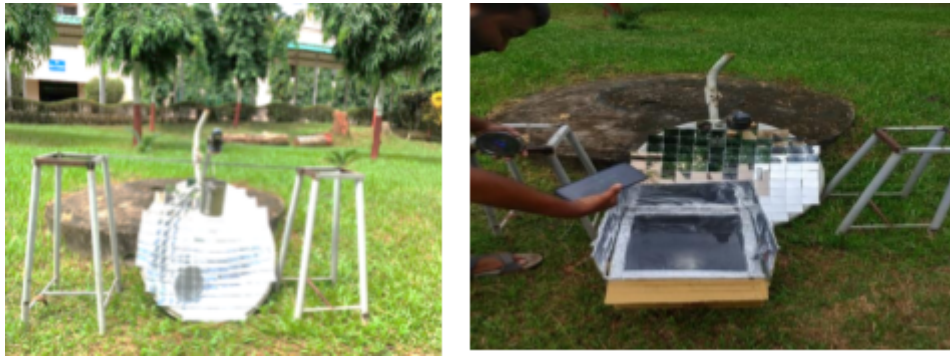
Figure: (a) Parabolic solar cooker (b) Box solar cooker
